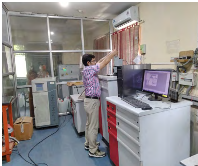
Running electrical measurements in a CCR (left) and magnetic measurements in a SQUID magnetometer (right).
